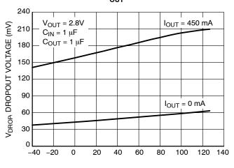
Figure 14. Dropout Voltage vs. Temperature - $V_{OUT} = 2.8 V$
