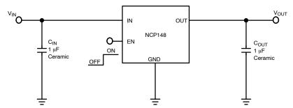
Figure 1. Typical Application Schematics
