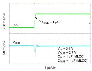
Figure 33. Load Transient Response – 1 mA to 450 mA – V<sub>OUT</sub> = 2.7 V
