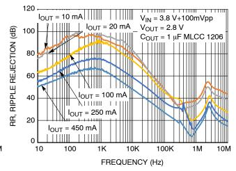
Figure 24. PSRR for Various Output Currents,  $V_{OUT} = 2.8 \text{ V}$
