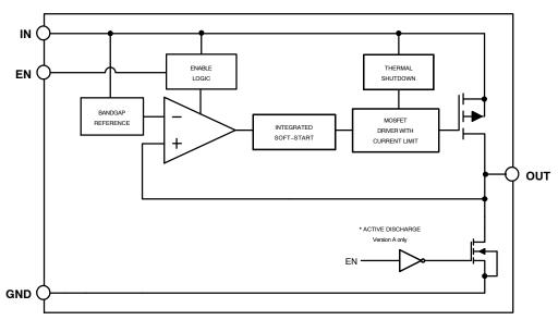
Figure 2. Simplified Schematic Block Diagram
