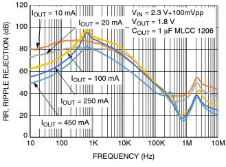
Figure 23. PSRR for Various Output Currents,  $V_{OUT}$  = 1.8 V
