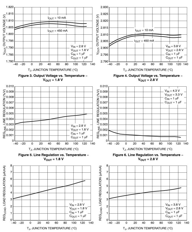
Figure 7. Load Regulation vs. Temperature –  $V_{OUT} = 1.8 \text{ V}$
