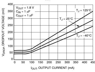
Figure 11. Dropout Voltage vs. Load Current -**V<sub>OUT</sub>** = 1.8 **V**
