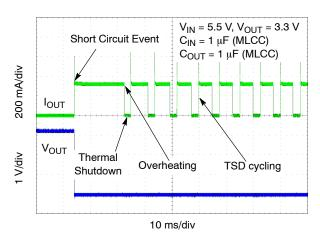
Figure 35. Short Circuit and Thermal Shutdown
