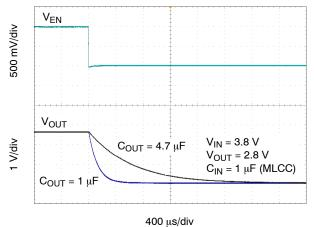
Figure 36. Enable Turn-Off (Active Discharge)
