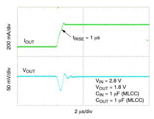
Figure 31. Load Transient Response – 1 mA to 450 mA – V<sub>OUT</sub> = 1.8 V
