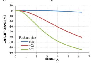
Figure 37. Capacity vs DC Bias Voltage
