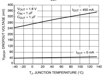
Figure 13. Dropout Voltage vs. Temperature -**V<sub>OUT</sub>** = 1.8 **V**
