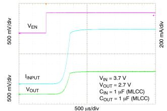
Figure 27. Enable Turn-on Response –  $C_{OUT}$  = 1  $\mu$ F,  $I_{OUT}$  = 10 mA
