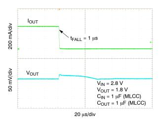
Figure 32. Load Transient Response – 450 mA to 1 mA – V<sub>OUT</sub> = 1.8 V
