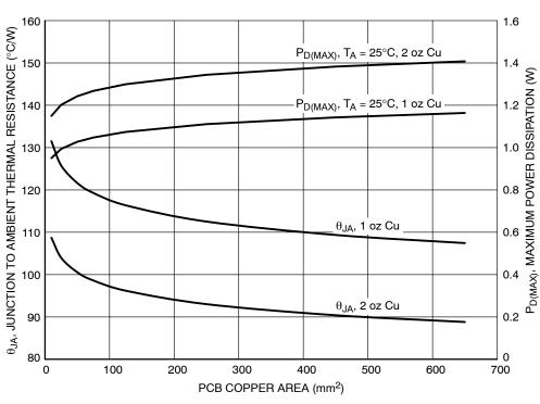
Figure 38.  $\theta_{JA}$  and  $P_{D \text{ (MAX)}}$  vs. Copper Area (CSP4)
