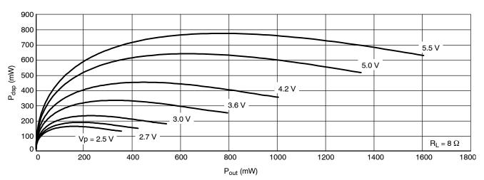
Figure 23. Power Dissipation vs. Pout
