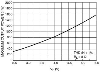
Figure 24. Maximum Output Power vs. V<sub>P</sub>
