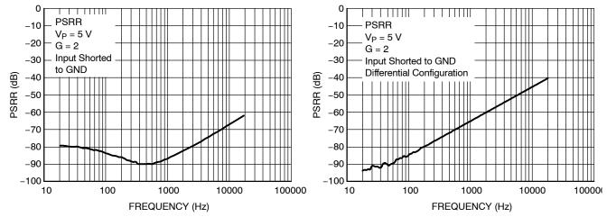
Figure 21. PSRR vs. Frequency
