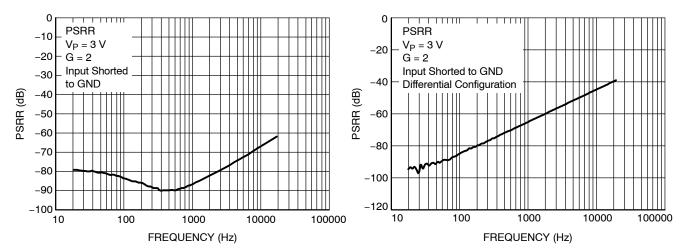
Figure 17. PSRR vs. Frequency
