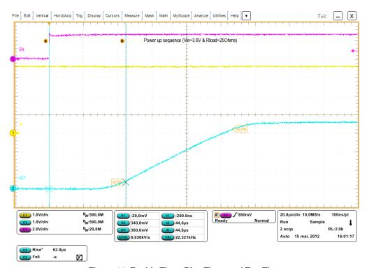
Figure 11. Enable Time, Rise Time, and Ton Time
