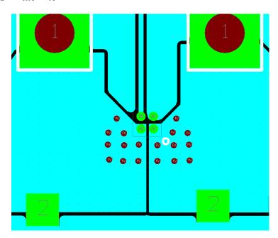
Figure 13. Routing Example 1 oz, 2 Layers, 100°C/W
