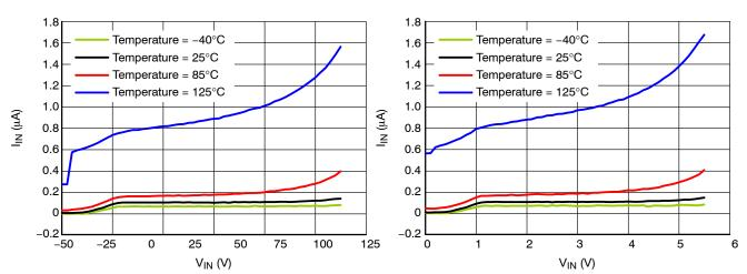
Figure 8. Standby Current ( $\mu A$ ) versus  $V_{IN}$  (V), No Load
