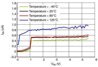
Figure 10. Quiescent Current ( $\mu$ A) versus V<sub>IN</sub> (V), No load.
