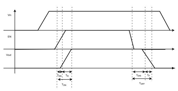
Figure 3. Enable, Rise and fall time
