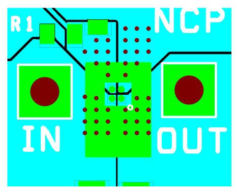
Figure 14. Routing Example 2 oz, 4 Layers, 60°C/W
