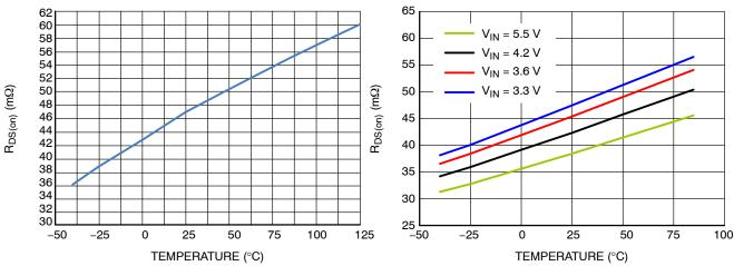
Figure 6.  ${\rm R_{DS(on)}}~({\rm m}\Omega)$  vs. Temperature (°C) at 3.3 V, Iload 100 mA
