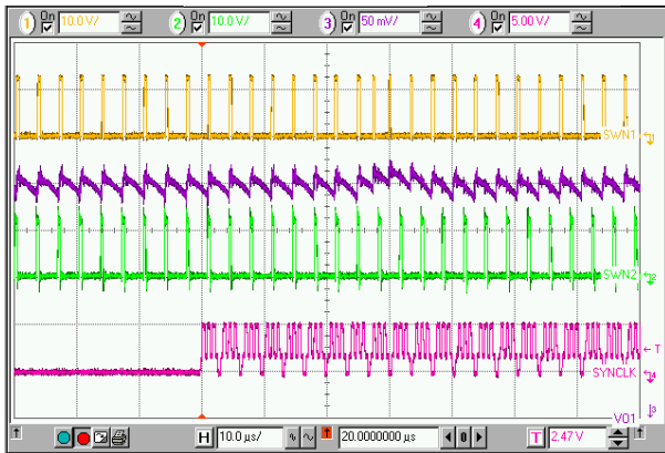
Top to Bottom: SWN_Slave, Vo_Slave, SWN_Master, Sync_clk
