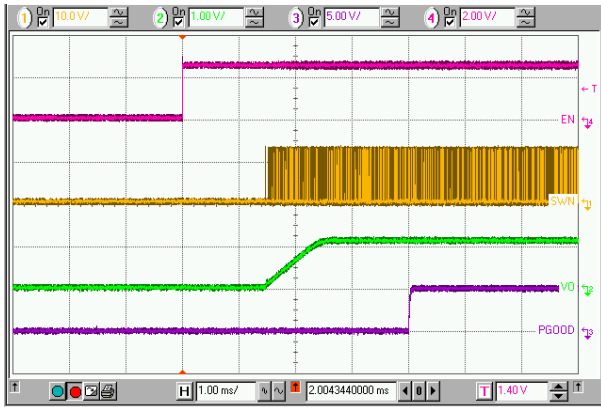
Top to Bottom: EN, SWN, Vo, PGOOD Figure 10. Powerup Sequence
