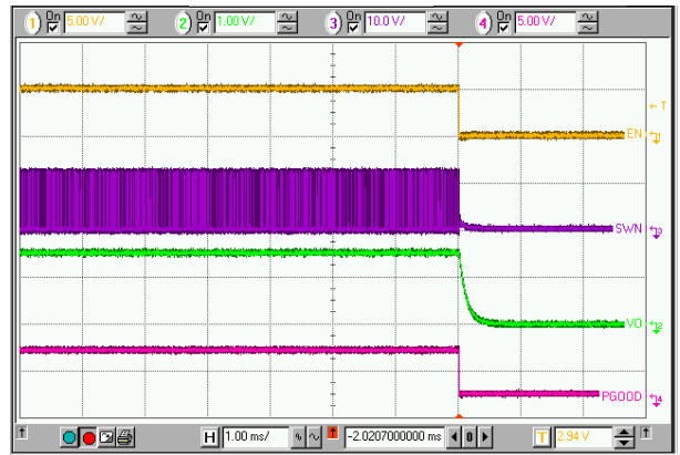
Top to Bottom: EN, SWN, V O , PGOOD Figure 10. Powerdown Sequence
