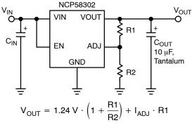
Figure 18. Adjustable Voltage Operation
