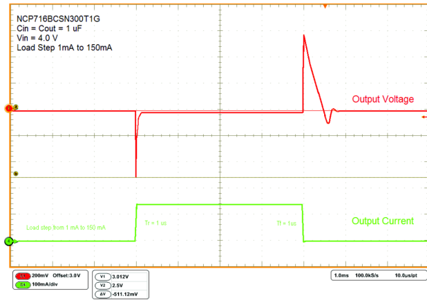
Figure 17. Load Transient Response
