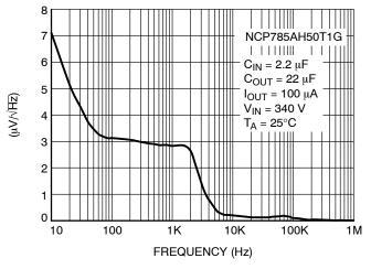
Figure 21. Output Noise Density vs. Frequency
