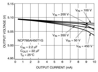
Figure 15. Output Voltage vs. Output Current
