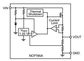
Figure 2. Simplified Internal Block Diagram
