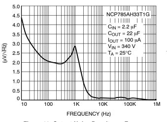
Figure 19. Output Noise Density vs. Frequency
