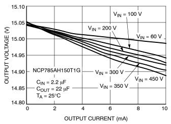
Figure 17. Output Voltage vs. Output Current
