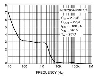
Figure 20. Output Noise Density vs. Frequency
