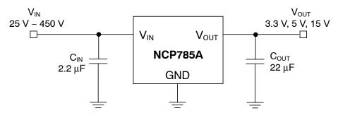
Figure 23. Typical Application Schematic
