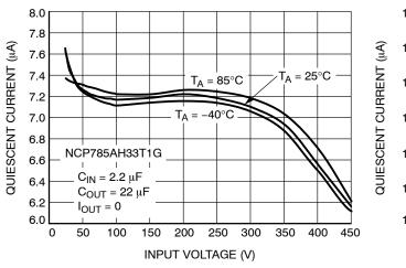
Figure 11. Quiescent Current vs. Input Voltage
