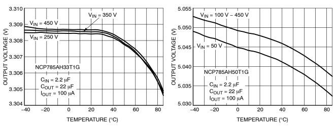
Figure 3. Output Voltage vs. Temperature
