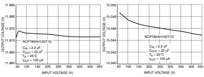
Figure 9. Output Voltage vs. Input Voltage
