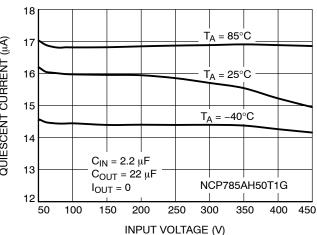
Figure 12. Quiescent Current vs. Input Voltage
