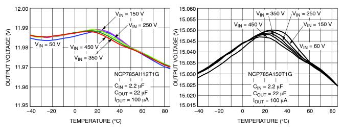
Figure 5. Output Voltage vs. Temperature
