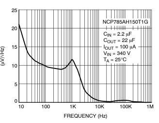
Figure 22. Output Noise Density vs. Frequency
