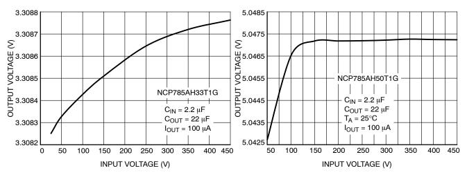
Figure 7. Output Voltage vs. Input Voltage
