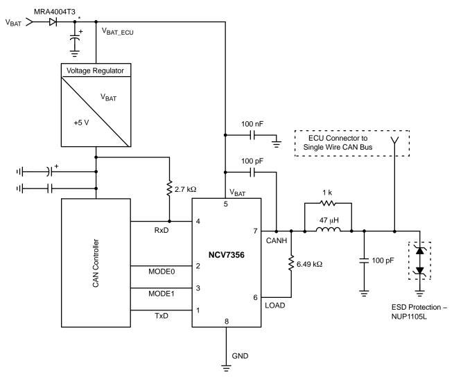
\*Recommended capacitance at  $V_{\mbox{\footnotesize{BAT\_ECU}}}\!>1.0~\mu\mbox{F}$  (immunity to ISO7637/1 test pulses)
