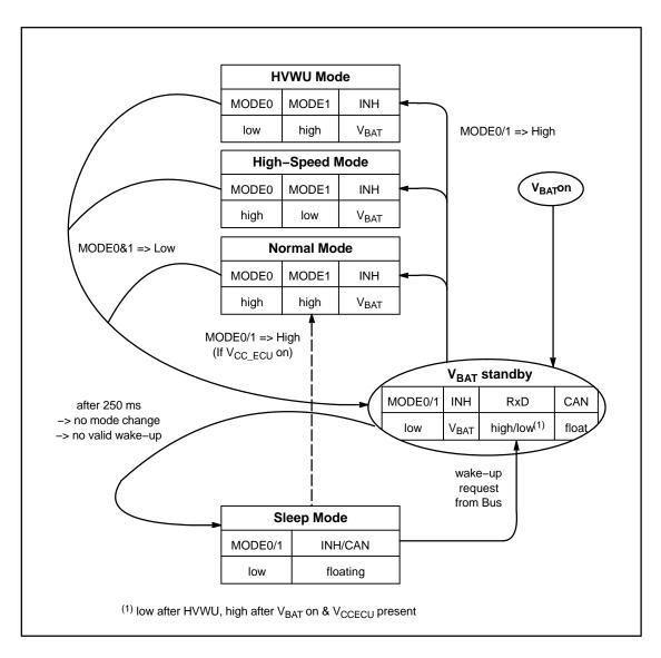
Figure 10. State Diagram, 14 Pin Package
