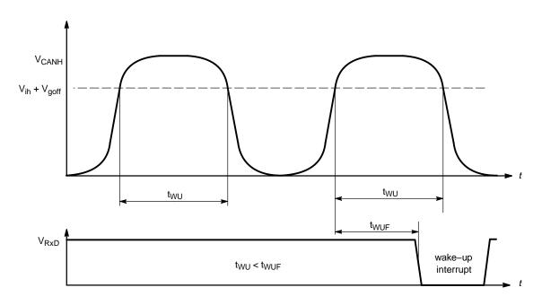
Figure 7. Wake-Up Filter Time Delay
