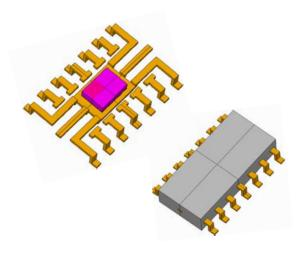
Figure 20. Internal construction of the package simulation.
