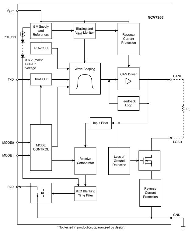
Figure 1. 8-Pin Package Block Diagram
