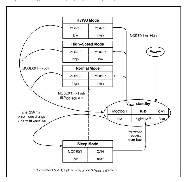
Figure 9. State Diagram, 8 Pin Package
