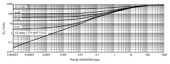
Figure 26. SOIC-14 Thermal Duty Cycle Curves on 1" Spreader Test Board
