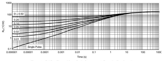
Figure 19. SOIC-8 Thermal Duty Cycle Curves on 1" Spreader Test Board
