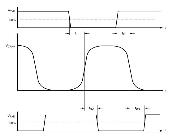
Figure 6. Input/Output Timing
