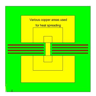
Figure 14. Min pad is shown as the red traces.
