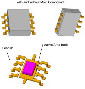
Figure 13. Internal construction of the package simulation.
