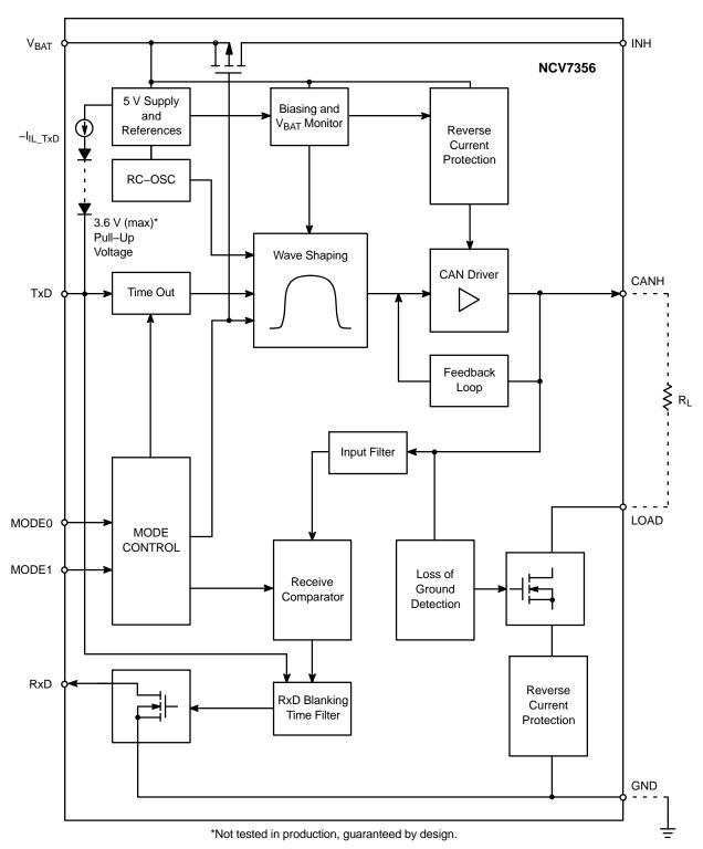
Figure 2. 14-Pin Package Block Diagram
