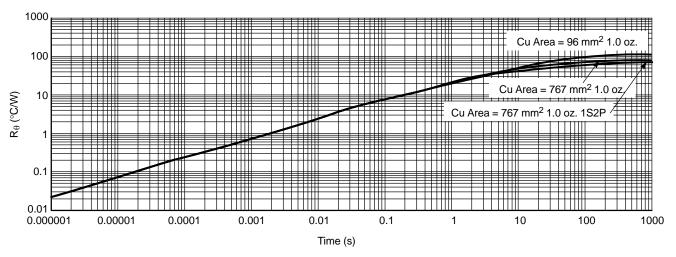
Figure 25. SOIC-14 Single Pulse Heating
