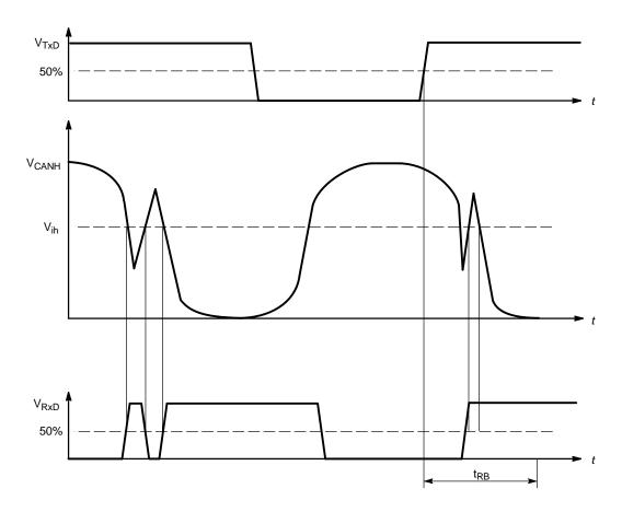
Figure 8. Receive Blanking Time
