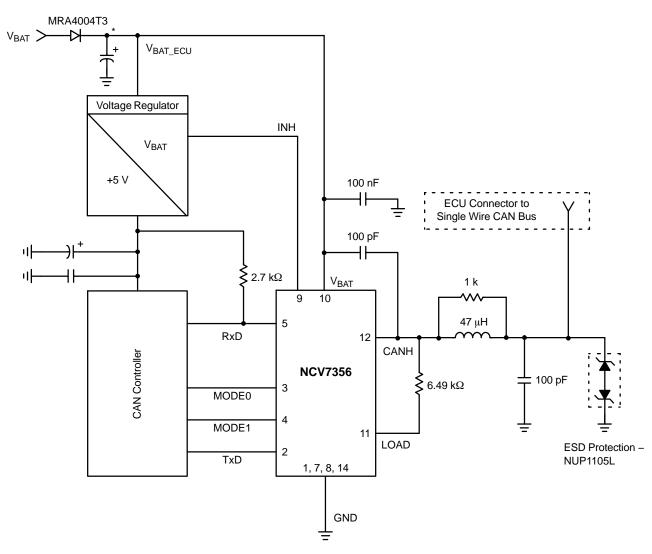
\*Recommended capacitance at  $V_{BAT\_ECU}$  > 1.0  $\mu F$  (immunity to ISO7637/1 test pulses)
