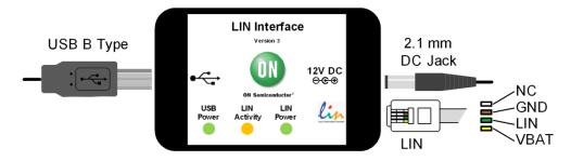
Figure 3. USB-LIN Interface Connectors
