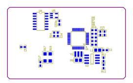
Figure 10. LIN Interface V3 Bottom Assembly Drawing
