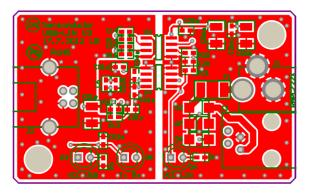
Figure 11. LIN Interface V3 PCB Top Composite Drawing
