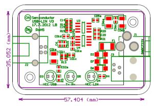
Figure 9. LIN Interface V3 Top Assembly Drawing
