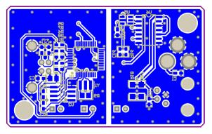
Figure 12. LIN Interface V3 PCB Bottom Composite Drawing
