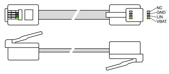
Figure 2. LIN Cable with RJ11 4P4C Connectors (Top View and Side View)
