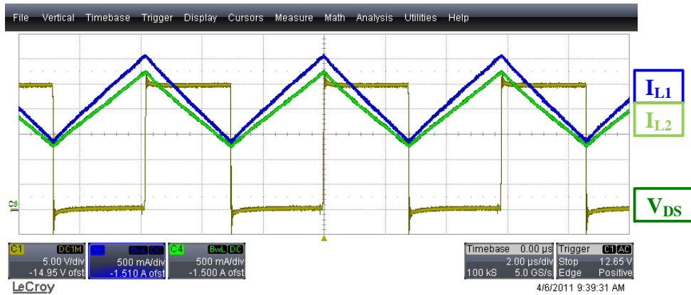
Figure 4. Operational Waveforms, V_{IN} = 12\text{ V} , R_{OUT} = 6\ \Omega
