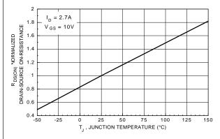
Figure 3. On-Resistance Variation with Temperature.
