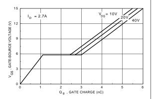
Figure 10. Gate Charge Characteristics.
