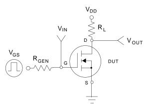
Figure 11. Switching Test Circuit.
