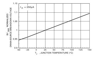
Figure 7. Breakdown Voltage Variation with Temperature.
