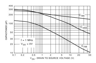
Figure 9. Capacitance Characteristics.
