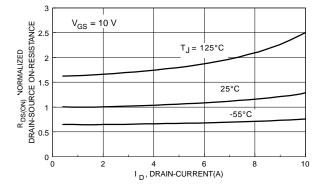
Figure 4. On-Resistance Variation with Drain Current and Temperature.
