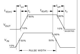
Figure 12. Switching Waveforms.
