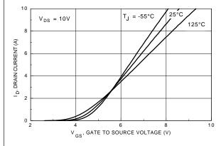
Figure 5. Transfer Characteristics.
