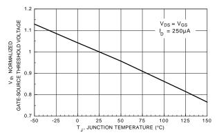
Figure 6. Gate Threshold Variation with Temperature.
