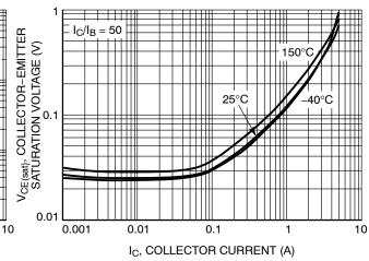
Figure 5. Collector-Emitter Saturation Voltage
