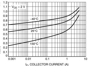
Figure 7. V<sub>BE(on)</sub> Voltage
