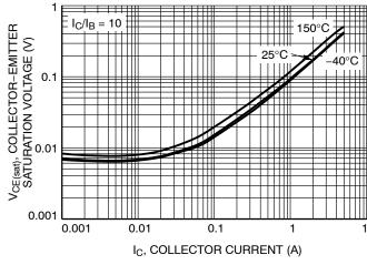
Figure 4. Collector-Emitter Saturation Voltage
