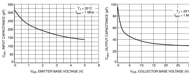
Figure 10. Input Capacitance
