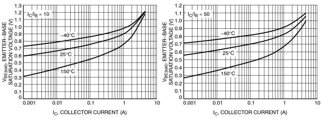
Figure 8. Base-Emitter Saturation Voltage
