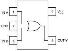
Figure 1. Pinout (Top View)
