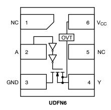
Figure 2. Pinout (Top View)
