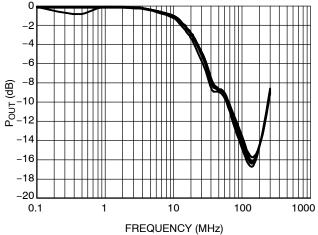
Figure 12. Bandwidth vs. Frequency @  $V_{CC}$  = 1.65 V to 3.6 V
