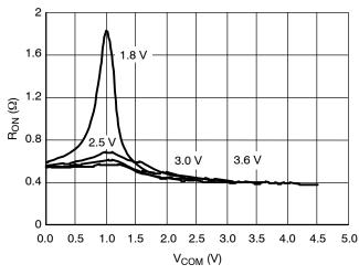
Figure 9. On-Resistance vs. COM Voltage
