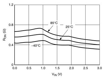
Figure 10. R<sub>ON</sub> vs. V<sub>IN</sub> vs. Temperature @ V<sub>CC</sub> = 3.0 V
