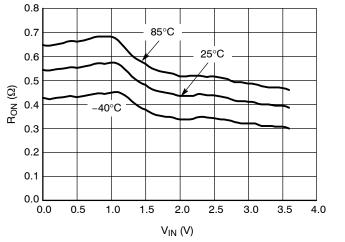
Figure 11. R<sub>ON</sub> vs. V<sub>IN</sub> vs. Temperature @ V<sub>CC</sub> = 3.6 V
