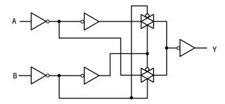
Figure 3. Expanded Logic Diagram (1/4 of Device)
