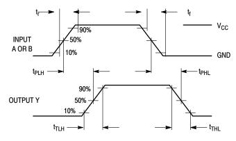
Figure 1. Switching Waveforms
