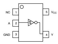
Figure 1. Pinout
