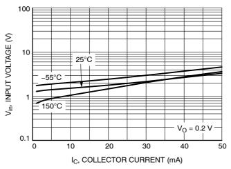
Figure 6. Input Voltage vs. Output Current
