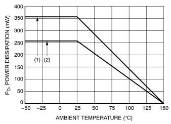
Figure 1. Derating Curve
