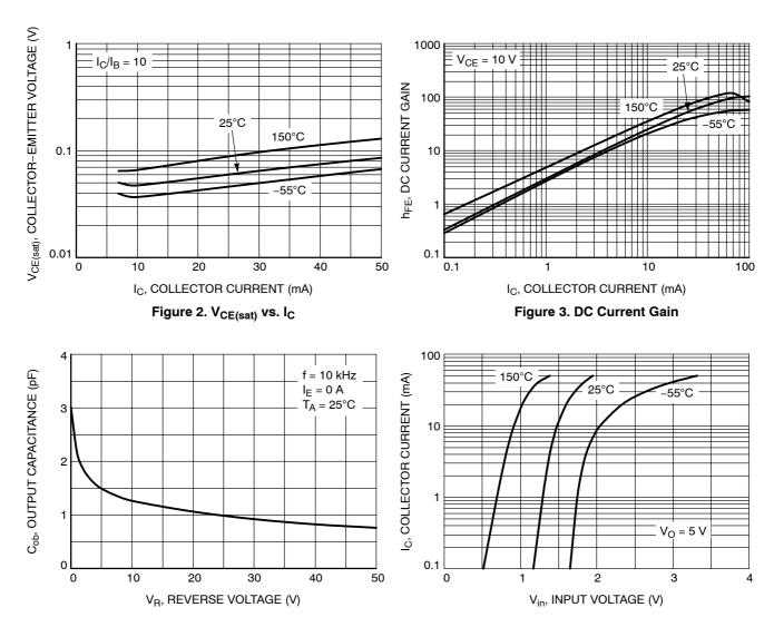
Figure 4. Output Capacitance
