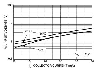
Figure 16. Input Voltage vs. Output Current
