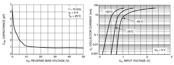
Figure 19. Output Capacitance
