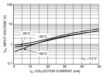
Figure 21. Input Voltage vs. Output Current
