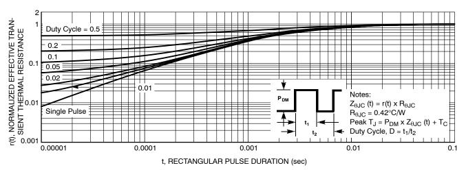
Figure 13. Junction-to-Ambient Transient Thermal Response Curve
