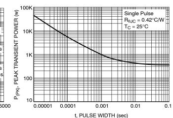
Figure 12. Single Pulse Maximum Power Dissipation
