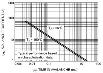
Figure 9. Unclamped Inductive Switching Capability
