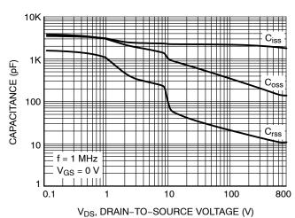
Figure 8. Capacitance vs. Drain-to-Source Voltage
