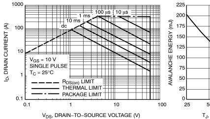
Figure 11. Maximum Rated Forward Biased Safe Operating Area
