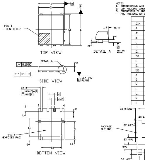
NDTES: 1. DIMENSIONING AND TOLERANCING PER ASME Y14.5M, 2009. 2. CONTROLLING DIMENSION: MILLIMETERS 3. DIMENSIONS DI AND E1 DO NOT INCLUDE MOLD FLASH, PROTRUSIONS, DR GATE BURRS.
