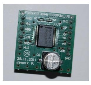
For the test of this DUT, the ON semiconductor evaluation kit for the AMIS\_306xx and ON Semi\_30627 has to be used. The procedure assumes that the test engineer is familiar with the use of the evaluation board and the GUI software.
