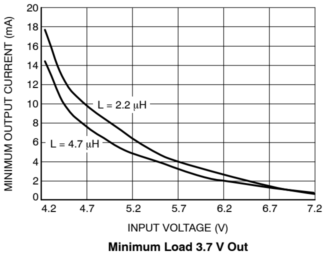
Figure 27. Minimum Load Current with Different Input and Output Voltages
