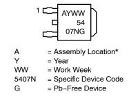
\* The Assembly Location code (A) is front side optional. In cases where the Assembly Location is stamped in the package, the front side assembly code may be blank.
