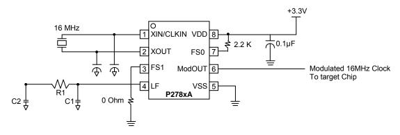
Note: Both logic input pins FS1 and FS0 have to be connected to either VDD or VSS. Do not leave them floating.
