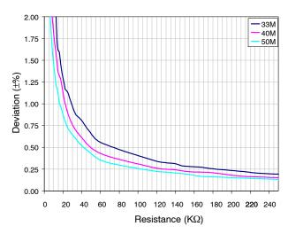
Figure 9. Deviation vs. Resistance (FS = 1, MR = 1)
