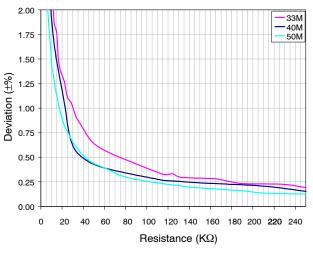
Figure 8. Deviation vs. Resistance (FS = 1, MR = 0)
