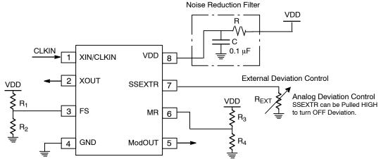
Note: FS (Pin#3) MR (Pin#6): Connect to VDD or GND Refer to Pin Description table for Functionality details.
