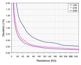
Figure 6. Deviation vs. Resistance (FS = 0, MR = 0)
