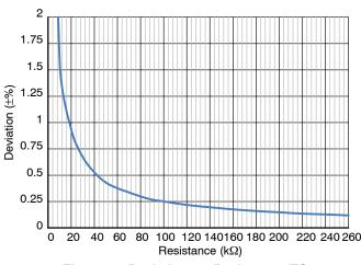
Figure 10. Deviation vs. Resistance (FS = 1, MR = 0)  $V_{DD} = 3.3 \text{ V}$
