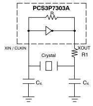
$C_X=2^{\star}(C_P-C_S),$  Where  $C_P=$  Load capacitance of crystal from crystal vendor datasheet.
