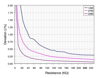
Figure 7. Deviation vs. Resistance (FS = 0, MR = 1)
