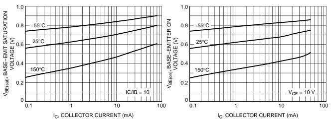
Figure 3. Base-Emitter Saturation Voltage
