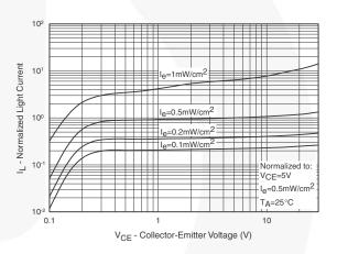
Figure 3. Dark Current vs. Collector - Emitter Voltage Figure 4. Light Current vs. Collector - Emitter Voltage
