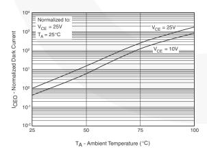
Figure 5. Dark Current vs. Ambient Temperature
