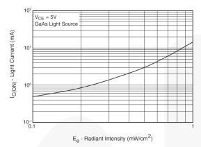
Figure 1. Light Current vs. Radiant Intensity
