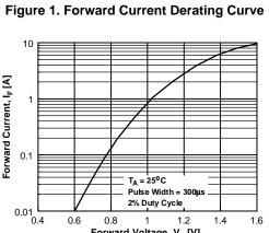
Figure 3. Forward Voltage Characteristics
