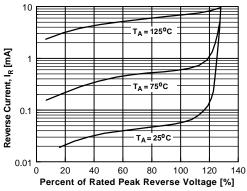
Figure 4. Reverse Current vs Reverse Voltage
