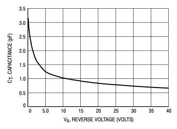
Figure 3. Typical Capacitance
