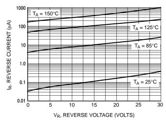
Figure 3. Leakage Current
