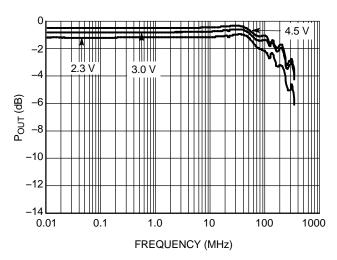
Figure 15. Bandwidth vs. Frequency
