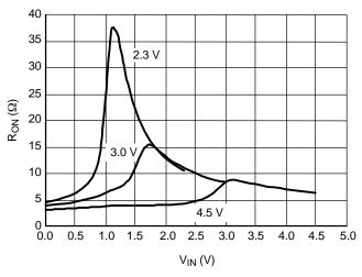
Figure 14. On-Resistance vs. Input Voltage
