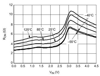
Figure 13.  $R_{ON}$  vs.  $V_{IN}$  vs. Temperature @  $V_{CC}$  = 4.5 V
