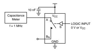
Figure 9. Channel On Capacitance
