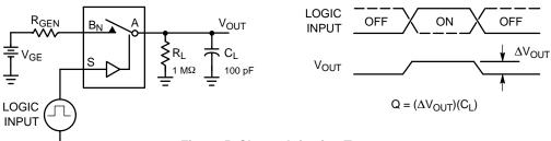
Figure 5. Charge Injection Test
