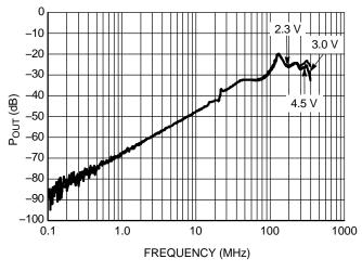
Figure 16. Off-Isolation vs. Frequency
