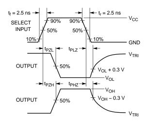
Figure 3. AC Waveforms
