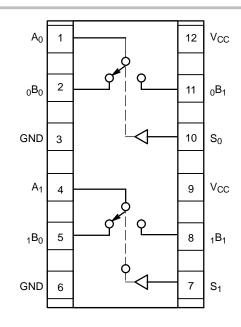
Figure 1. Pinout (Top View)
