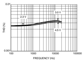
Figure 11. Total Harmonic Distortion vs. Frequency
