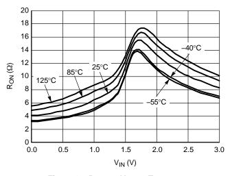
Figure 12.  $R_{ON}$  vs.  $V_{IN}$  vs. Temperature @  $V_{CC}$  = 3.0 V
