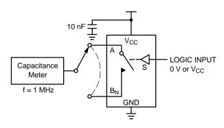
Figure 8. Channel Off Capacitance
