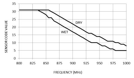
Figure 2. Sensor Code for Wet and Dry Conditions
