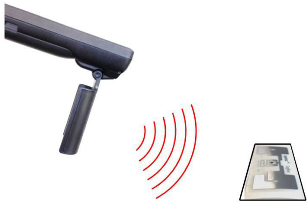
Figure 10. Proper Reader Antenna and Tag Orientation
