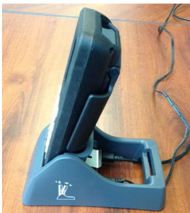
Figure 1. Connecting the Reader to the Cradle
