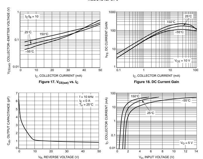
Figure 19. Output Capacitance
