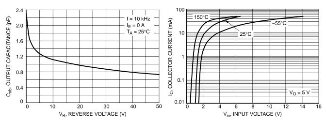
Figure 14. Output Capacitance
