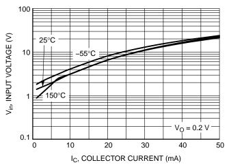
Figure 21. Input Voltage vs. Output Current
