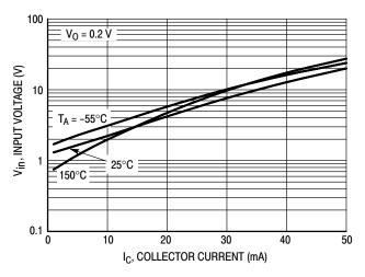
Figure 6. Input Voltage vs. Output Current
