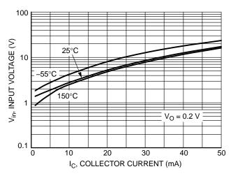
Figure 16. Input Voltage vs. Output Current
