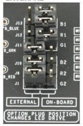
Pinout for external connections are Vin (12V provided), Green PWM, Red PWM, Blue PWM
