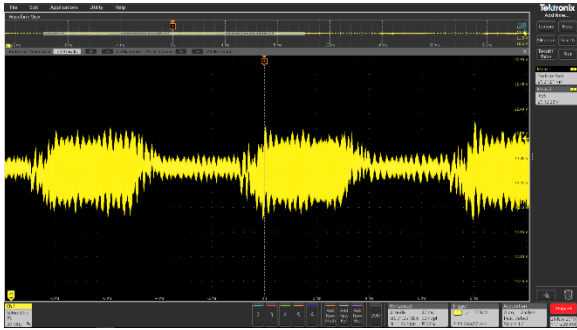
Figure 20 - Transient load on 12V VBUS
