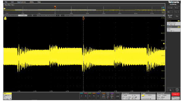
Figure 19 - Transient load on 9V VBUS
