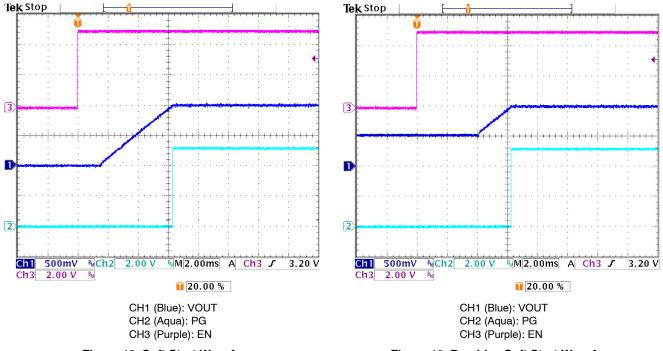
Figure 18. Soft Start Waveform (Vin = 12 V, Vout = 1 V)
