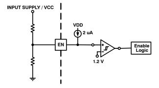
Figure 22. Enable Functional Block Diagram
