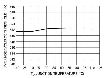
Figure 15. Output UVP vs. Junction Temperature
