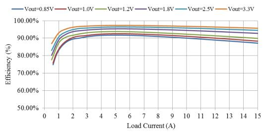
Figure 17. Efficiency vs. Load Current (Vin=5.5 V)
