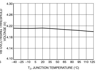
Figure 11. OTS Threshold vs. Temperature
