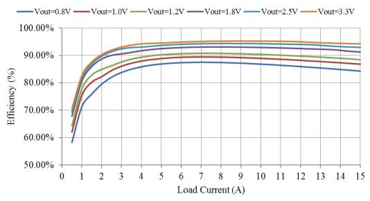
Figure 16. Efficiency vs. Load Current (Vin=12 V)
