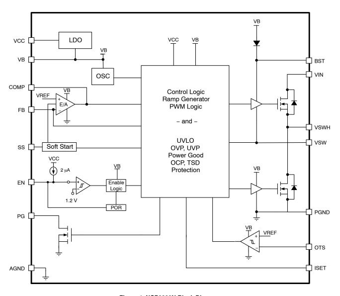
Figure 1. NCP3232N Block Diagram
