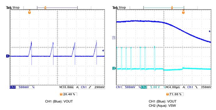
Figure 20. Output Voltage Hiccup Protection Waveform
