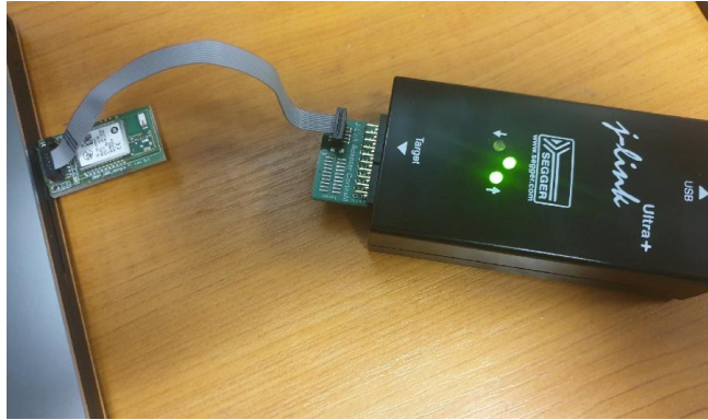
Figure 9: J-Link connection to USB Board
