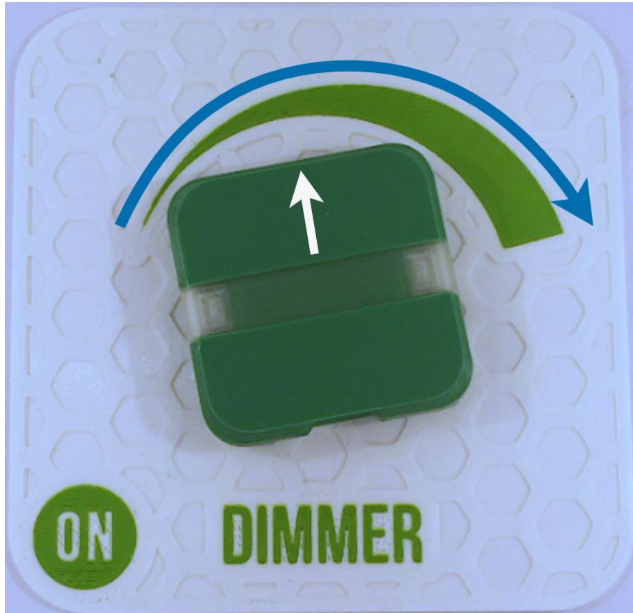
Figure 11: Mesh Node on dimmer pad showing range of operation
