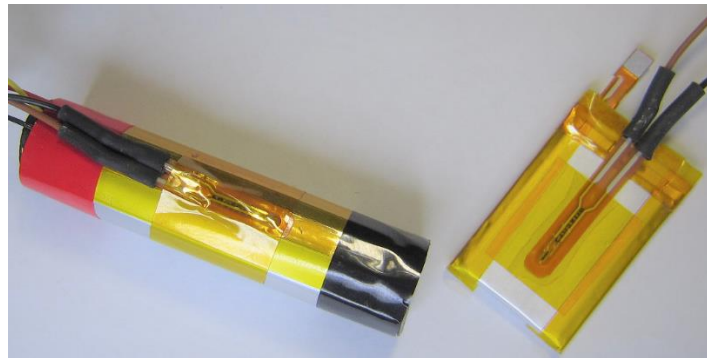
Figure 7. A LEAD TYPE THERMISTOR MOUNTING
