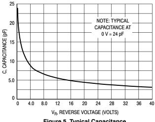
Figure 5. Typical Capacitance
