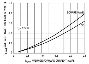
Figure 7. Power Dissipation
