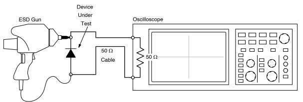
Figure 6. Diagram of ESD Clamping Voltage Test Setup
