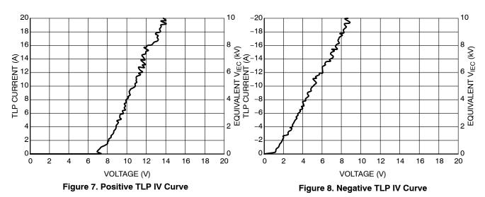
NOTE: TLP parameter:  $Z_0 = 50 \Omega$ ,  $t_p = 100 ns$ ,  $t_r = 300 ps$ , averaging window:  $t_1 = 30 ns$  to  $t_2 = 60 ns$ .
