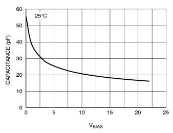
Figure 5. Capacitance vs.  $V_{\text{BIAS}}$
