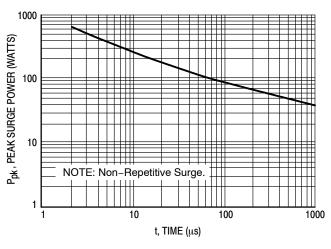
Figure 1. Peak Power Dissipation versus Pulse Width
