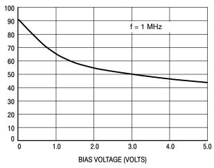
Figure 4. Junction Capacitance versus Reverse Voltage
