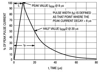
Figure 2. Pulse Waveform 8 x 20  $\mu$ s
