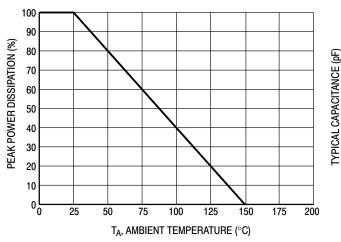
Figure 3. Power Derating Curve
