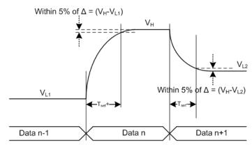
Figure 4. Output Settling Diagram
