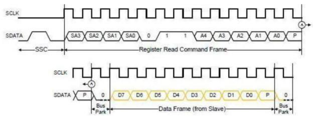
Figure 15. Register Read Command Sequence
