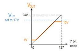
Figure 7. DAC Output Range Example A
