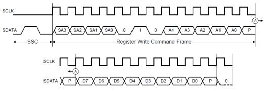
Figure 13. Register Write Command Sequence
