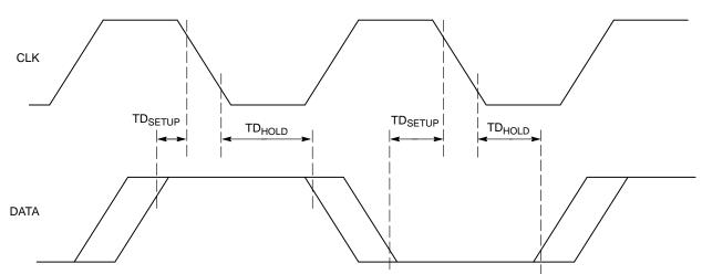
Figure 9. MIPI-RFFE Signal Timing during Master Writes to PTIC Control IC
