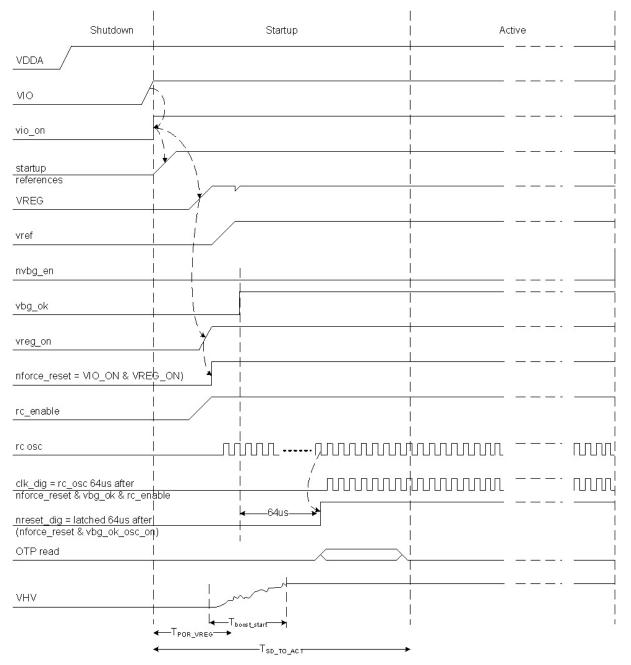
Figure 5. Startup Timing Diagram
