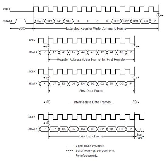
Figure 14. Extended Register Write Command Sequence
