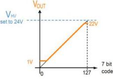
Figure 8. DAC Output Range Example B
