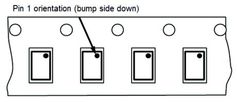
Figure 18. Orientation in Tape
