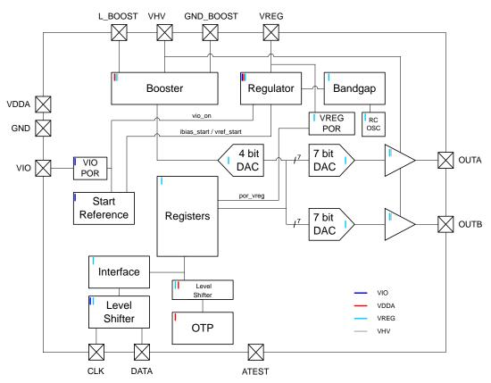
Figure 1. Control IC Functional Block Diagram
