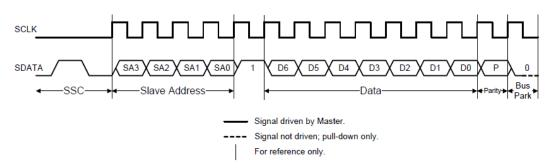
Figure 12. Register 0 Write Command Sequence
