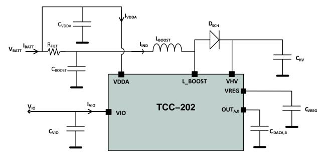
Figure 16. TCC-202 with External Components
