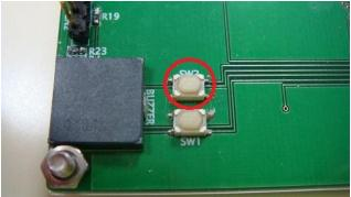
Figure 4: Reset Switch of MCU
