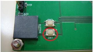
Figure 5: Reset Switch of LC717A10AR and LC898301XA
