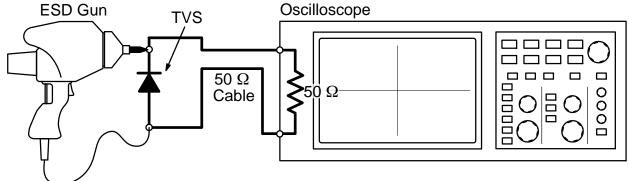
Figure 7. Diagram of ESD Test Setup
