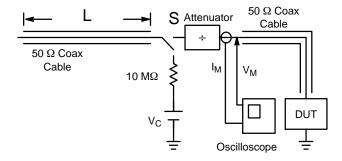
Figure 4. Simplified Schematic of a Typical TLP System
