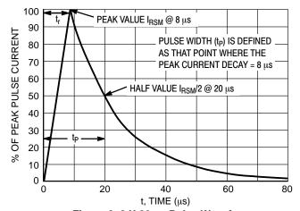
Figure 8. 8 X 20 µs Pulse Waveform
