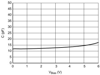
Figure 3. CV Characteristics
